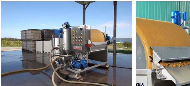
A lees filter helps the winery capture every luscious drop of juice. (see pg.107 )
