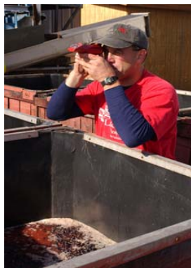
Winemaker tests for Brix with a refractometer.
